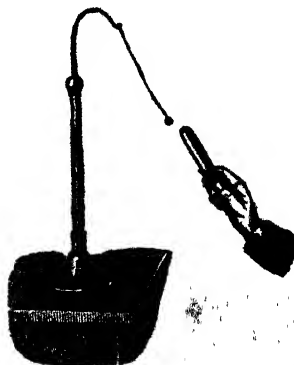
FIG. 74. A pith-ball hung by a silk string is repelled by an electrified stick of sealing-wax, or glass.
